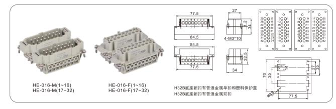
工作电流: 16A 工作电压: 400/500V 阻燃等级(据UL94): V0 防护等级: IP65 接线形式:螺钉压接 弹片压接 冷压针压接 电缆入口可选螺纹: M32, PG29 Rated current: 16A Rated voltage: 400/500V Flammability acc. to UL94: V0 Degree of protection acc. to DIN40 050: IP65 Terminal: Screw terminal Spring terminal Crimp terminal
