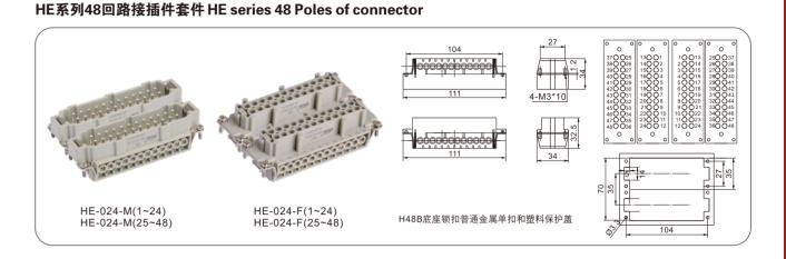
工作电流: 16A 工作电压: 400/500V 阻燃等级(据UL94): V0 防护等级: IP65 接线形式:螺钉压接 弹片压接 冷压针压接 电缆入口可选螺纹: PG29, PG36, M40 Rated current: 16A Rated voltage: 400/500V Flammability acc. to UL94: V0 Degree of protection acc. to DIN40 050: IP65 Terminal: Screw terminal Spring terminal Crimp terminal Thread: PG29, PG36, M40
